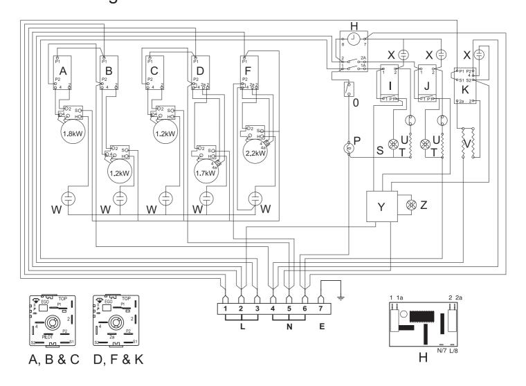
Connection shown in circuit diagram is for single phase. Ratings are for 230V 50Hz
